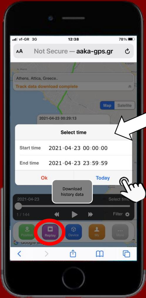
The Select time button, allows you to choose a specific date (from when to when) and a specific time ( from when to when)
